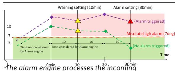
The alarm engine processes the incoming temperature data, according to the alarm configurations in Weboffice, and decides if an event (like a warning or an alarm) should be triggered or not.
